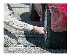
The first thing to do is to inspect the physical condition of all the tires, including the spare tyre. There should be no tears or bulges in the side walls. There should be a good amount of thread left on all the tyres. Next, you need to check if all the tyres are properly inflated as per the recommended levels of your car/vehicle. Keep in mind that the PSI levels that are printed on your tyres may not be most suitable for your specific make and model. Besides providing safety, properly
